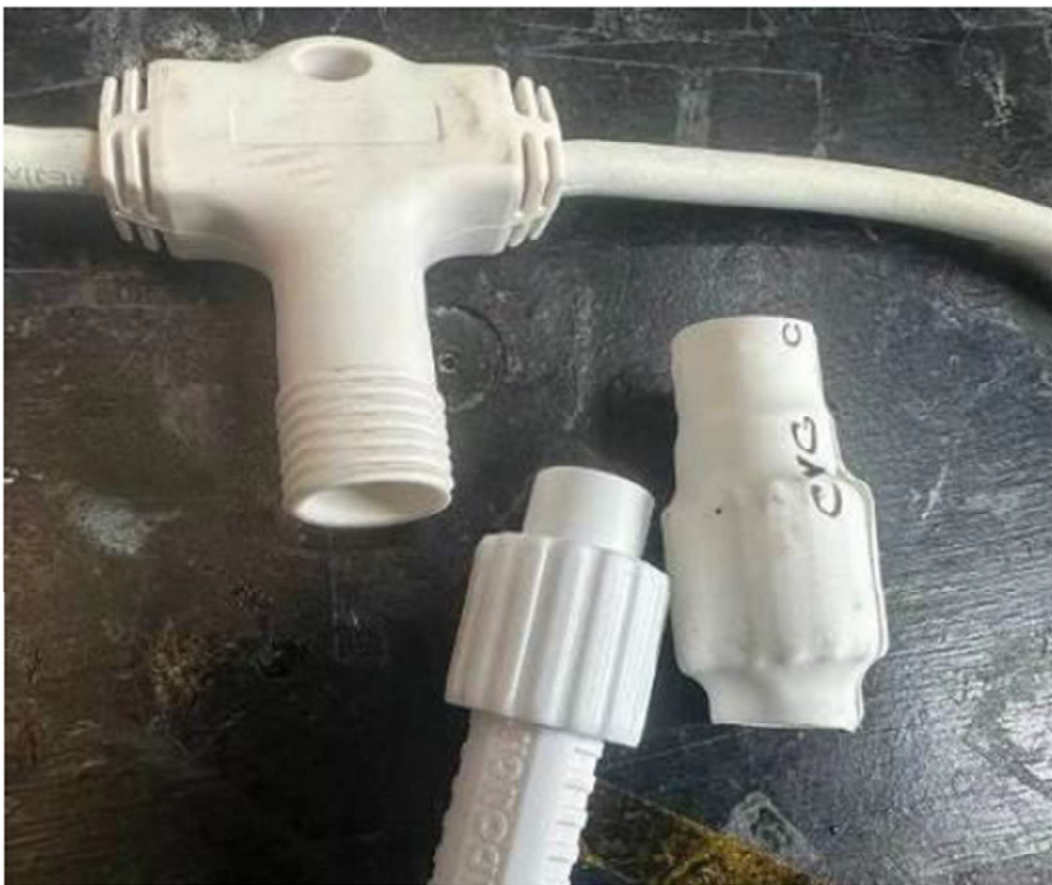
Female and male connector for branch connection (not connectable)
